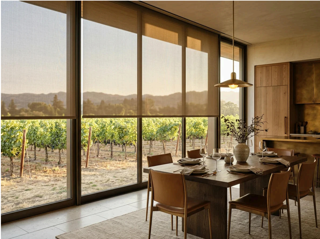
Mesh at half drop on a valley-floor dining room. The point of an open weave is that you can still see out — it is a glare tool, not a heat tool.
